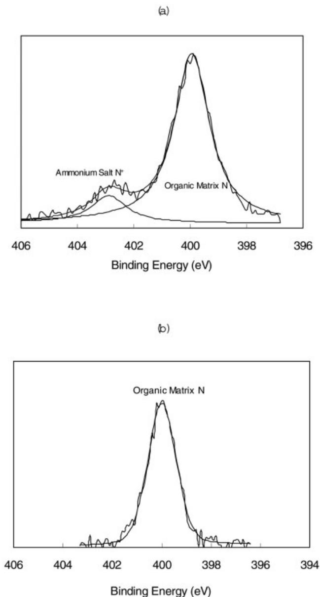
**Figure 5.** XPS N1s spectra of (a) microcomposite surface (T1C-20); (b) native HA.
