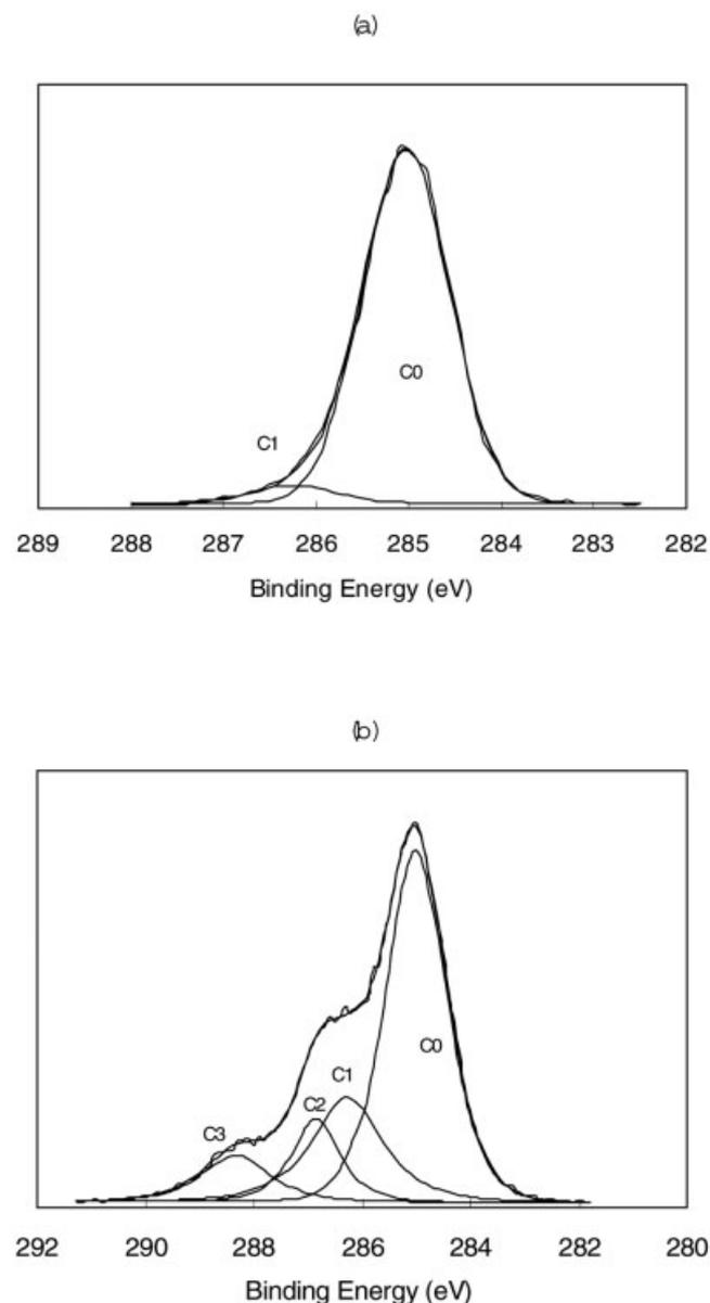
**Figure 6.** XPS C1s spectra of (a) UHMWPE preform and (b) microcomposite surface (T1C-20).
