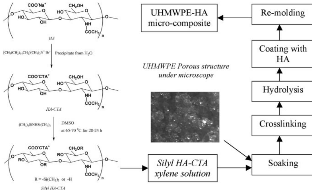
**Figure 1.** Formation of UHMWPE-HA microcomposite (with exception of those in Treatments-1A and -1B-see Table I).
